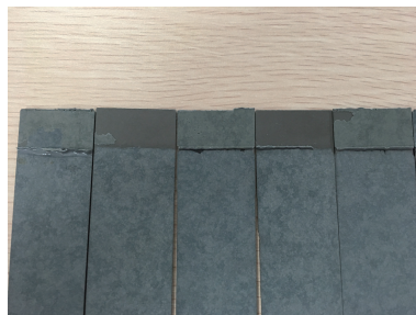
图6 微弧氧化剪切试样典型失效模式 Fig.6 Failure forms of micro-arc oxidation samples
